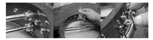
The bottom coordinator rod attaches in the same way. The bottom rod is longer and the shaft goes all the way through the hole in the wood rim first before you will be able to attach it to the bottom lag bolt. Don't worry, it isn't possible to do it backwards. I use this
