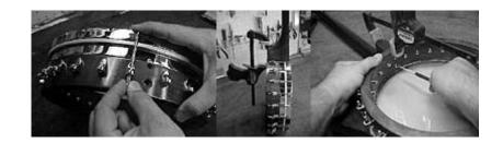
Install the 24 hooks and nuts and as shown starting on 4 imaginary compass points then filling the rest in and tighten the head down keeping the tension hoop parallel to the tone ring. Tightening each nut the same 1/4 turn even though they don't "feel" evenly tensioned this will help insure the head IS of an even tension. Tighten the head until it is reasonably close to the tension you would like it to be when the banjo is assembled.
